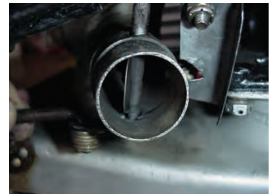
>> Bypass valve, shown here in the open position with carburetor heat selected off. Proper operation of this valve is critical for adequate heat if carburetor heat is selected on.
