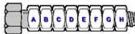
FIGURE 2 There is only one way to take this assembly apart, but more than 40,000 ways to put it back together.
