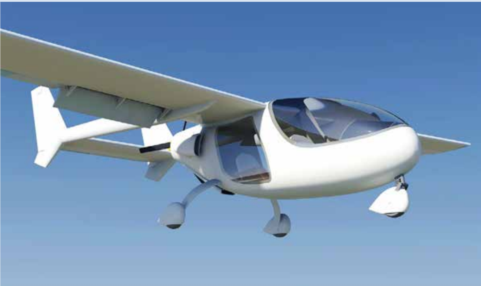
FIGURE 2 The current incarnation of my Project-Ex design has Slotted Flaps which should give an estimated 42kt stall speed when loaded to 600kg
