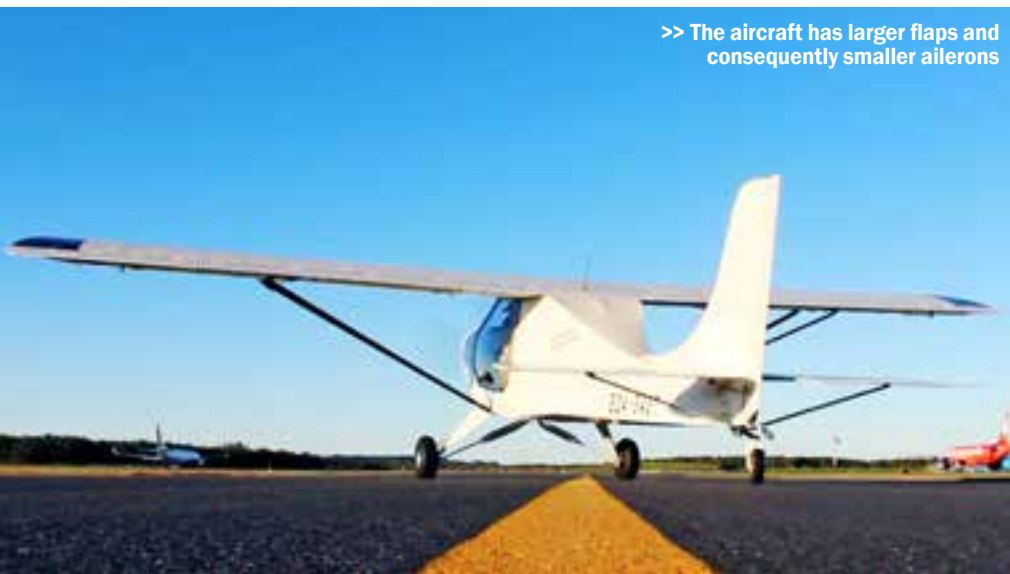
>> The GR-LSA has a different shaped and smaller wing
